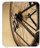
DERAILLEURS (named from the French word meaning 'derail') move the chain among two to six sprockets of different diameters to change gears.
