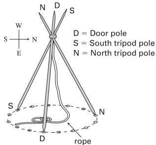
The diagram at the right shows a design for a 15-pole frame, in which three poles are erected first to form a tripod.
