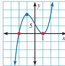
**Graph the polynomial function. Identify the  $x$ -intercepts and the points where the local maximums and local minimums occur.**
